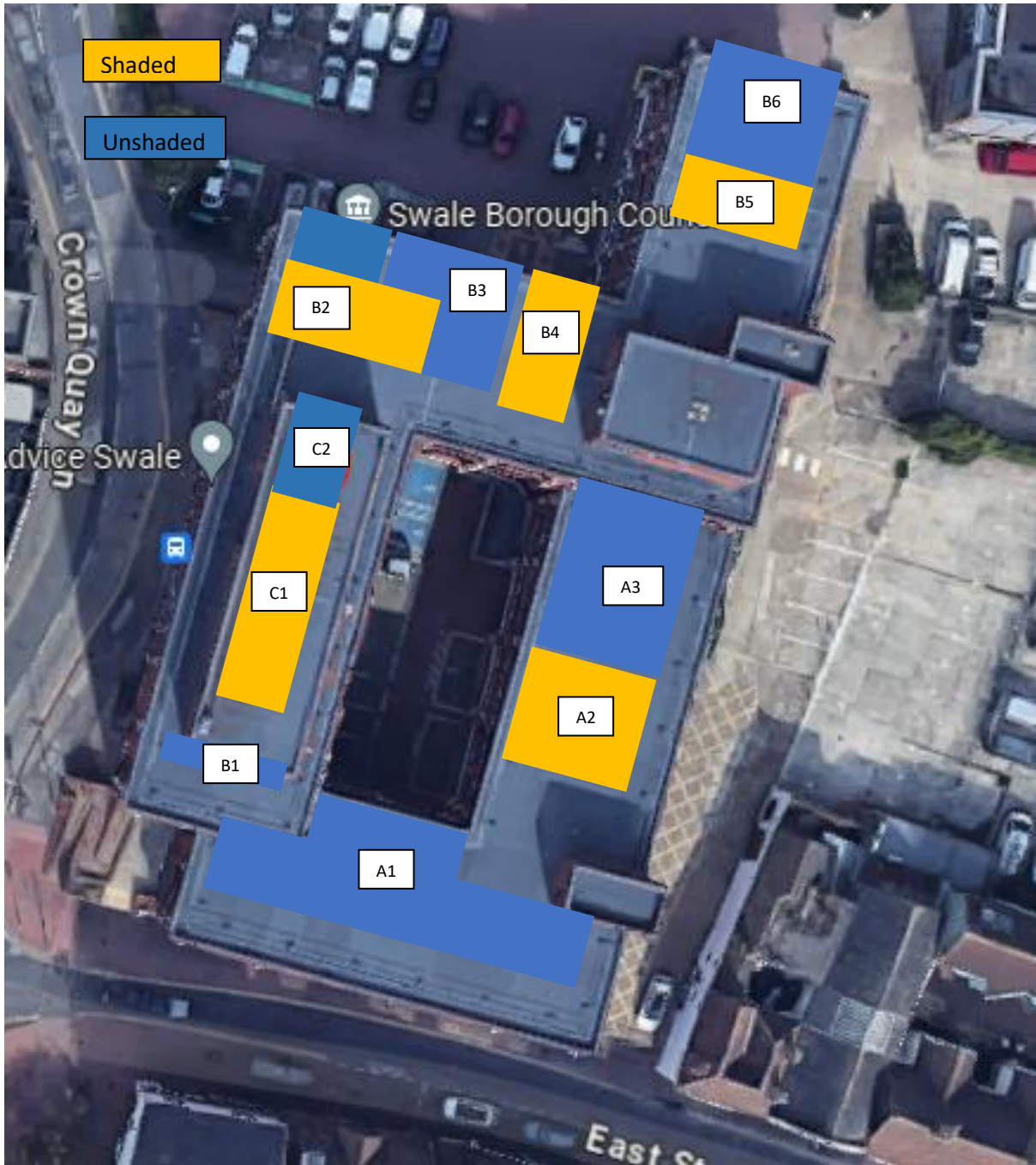
Figure 1 – Swale House Roof PV Layout
