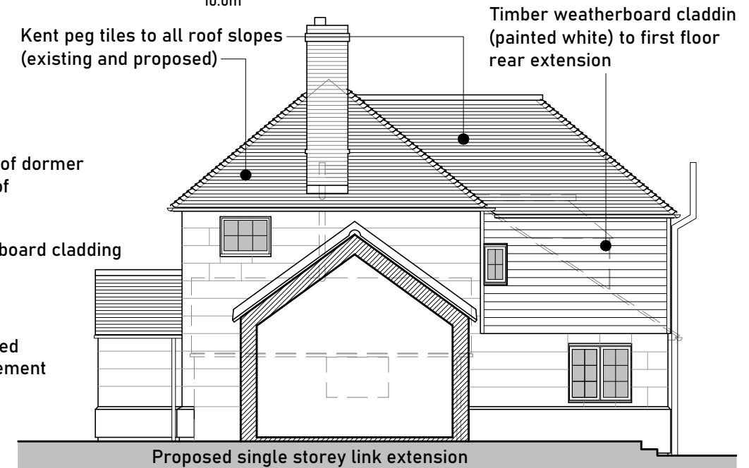
Side Elevation (North facing)
