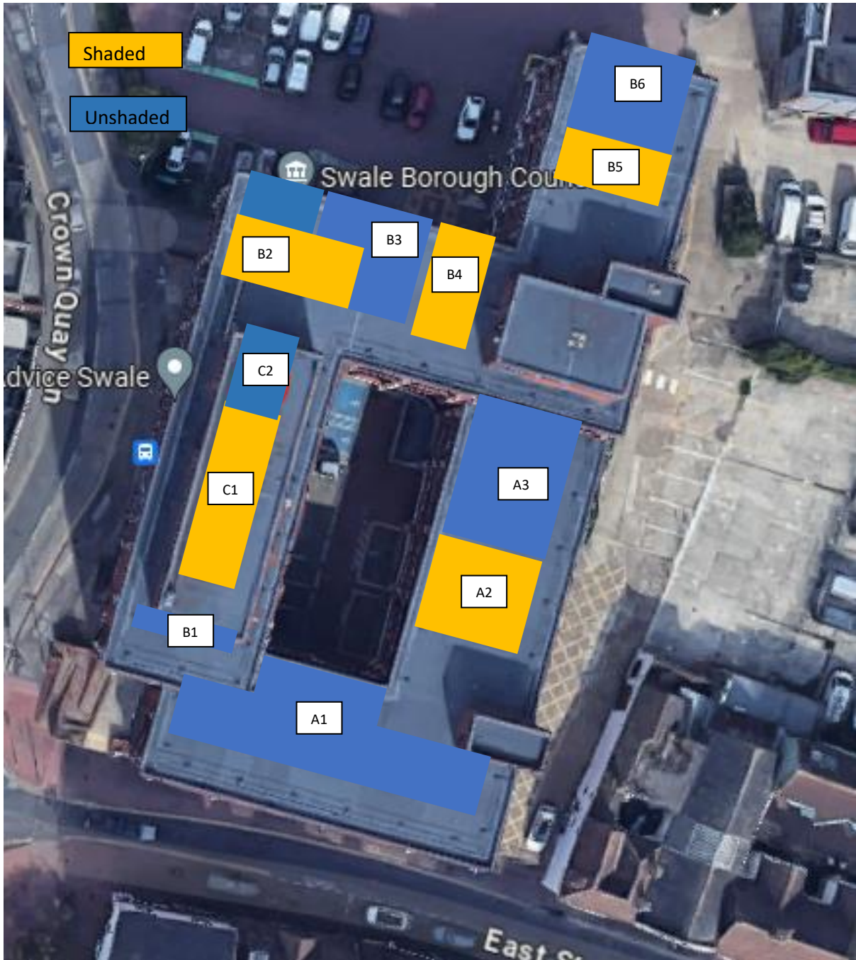
Figure 1 – Swale House Roof PV Layout
